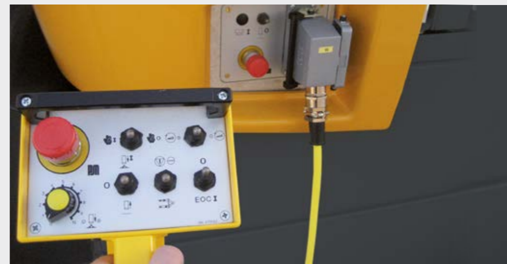
The radio remote control (optional) allows the machine to be controlled over long distances
