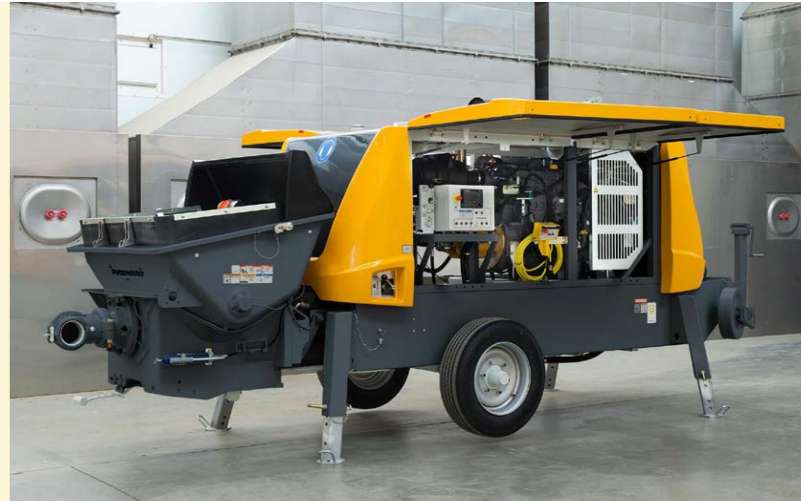
Swing doors, for example, ensure easy access, and protect the machine operator from rain and sun while working inside the machine
