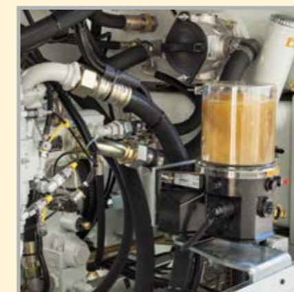
The electronic central lubrication system saves time and minimizes wear
